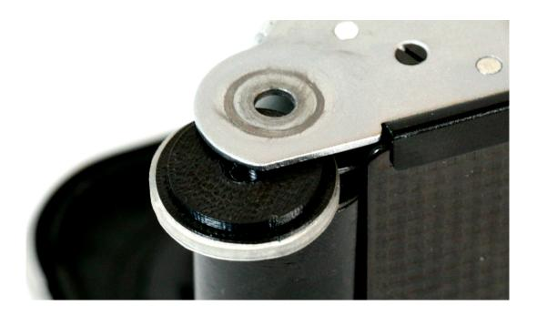
Step 4: Replace the sprocket wheel, turning it clockwise to thread into the all-perf wheel. Turn it until it stops; do not force it any further. It should stand up several millimeters above the back insert's top surface:
